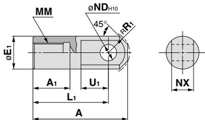
Material: Sulfur free-cutting steel
