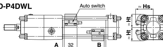
**Auto Switch Proper Mounting Position (Detection at Stroke End) and Mounting Height**
