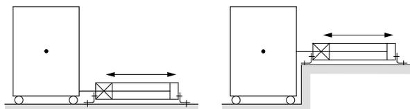
× Load center of gravity and cylinder shaft center are not matched.
