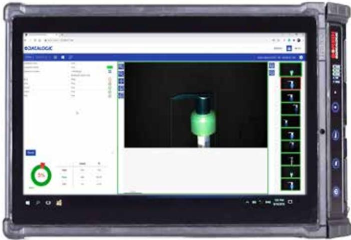
A new monitoring option added to CPM and SDK, the Smart Camera Monitor (SCM), provides immediate access to inspection results, statistics and parameters, image diagnostics to any devices able to run a web browser
